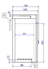
D Drain Electrical inlet (power) Refrigerant Outlet
